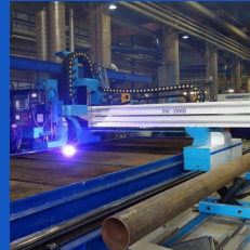
AMG – FSC 3500D CNC PLASMA CUTTER
