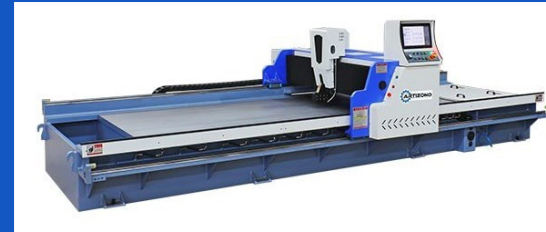
TANTAN CNC V-GROOVING MACHINE
